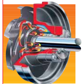
Advanced Technology 45° Conical Seal Chamber with integral flow modifiers redirects solids and slurry away from seal and back into the flow path of the process liquid, extending seal life and improving pump reliability.
